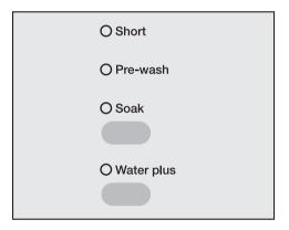
Press the appropriate additional option button. Press the top button repeatedly until the indicator light for the additional option you want comes on.
